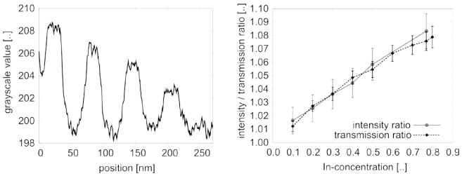
Fig. 2. a) Intensity linescan across the  $In_xG_{1-x}As/GaAs$  QW structure. b) Comparison of measured intensity ratios with simulated transmission ratios as a function of the In- concentration.
