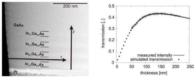
Fig. 1. a) HAADF STEM cross-section image of wedge-shaped sample at 25 keV. b) Comparison of the measured intensity along the GaAs layer with simulated electron transmission as a function the sample thickness.
