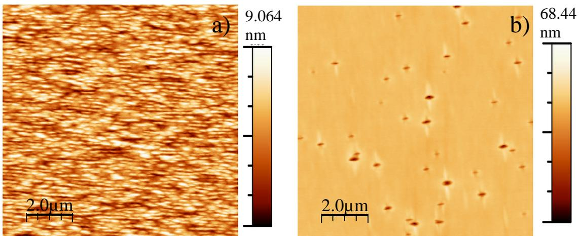
Fig. 2. AFM images of surfaces, a) without in-situ annealing, b) with annealing
