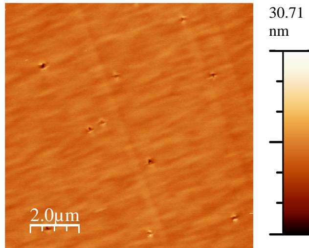
Fig. 3. AFM images of device surface with AlAs layers
