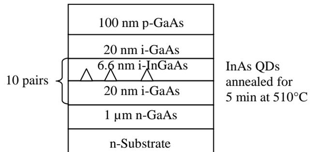
Fig. 1. Device structure.
