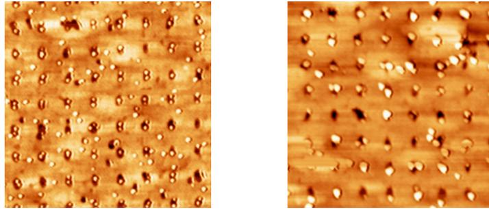
Fig. 1: AFM images ( $2\ \mu\text{m} \times 2\ \mu\text{m}$ ) of two samples with InAs QDs grown on patterned GaAs substrates; as grown (left), annealed (right).
